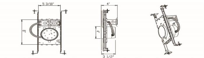
The DN-04S-GU is designed for use in non-insulated celling or for insulated celling but insulation must be kept 3" from all sides of the housing.
