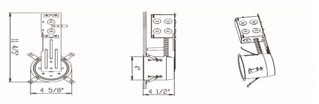
The DN-05S-GU is designed for use in non-insulated celling or for insulated celling but insulation must be kept 3" from all sides of the housing.
